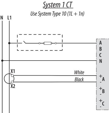
*Diagram 2: 1-Phase Line-to-Line 2-Wire*
