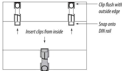
3. To reduce horizontal shifting across the DIN rail, use two Veris AV02 end stop clips.
