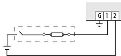
DC Control Power from 125 VDC to 300 VDC (UL and CE max.)
