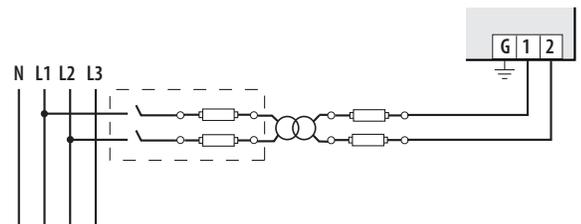
The Control Power Transformer may be wired L-N or L-L. Output to meet meter input requirements
