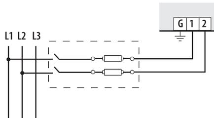
Line to Line from 90 VAC to 600 VAC (UL) (520 VAC for CE). In UL installations the lines may be floating (such as a delta). If any lines are tied to an earth (such as a corner grounded delta), see the Line to Neutral installation limits. In CE compliant installations, the lines must be neutral (earth) referenced at less than 300 VAC<sub>L-N</sub>
