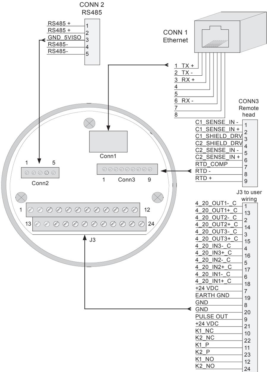
Fig. 19 Wiring connections are summarised in the following figure
