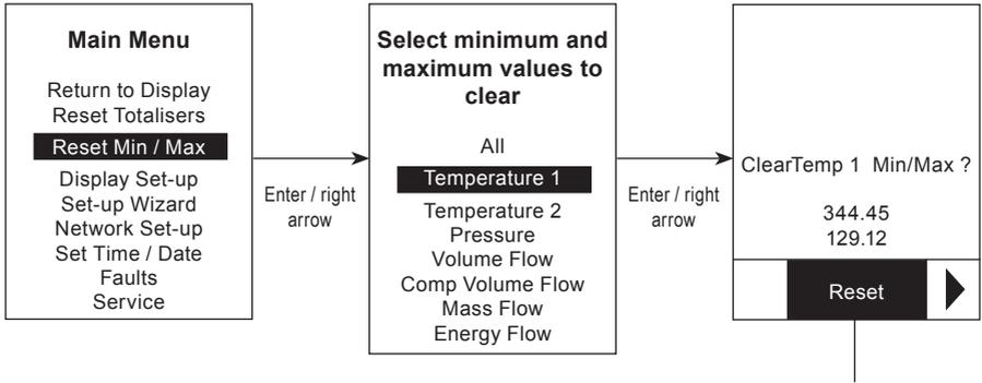
Use the right arrow key to select the middle field. The word 'Reset' appears to indicate this parameter can be reset.
