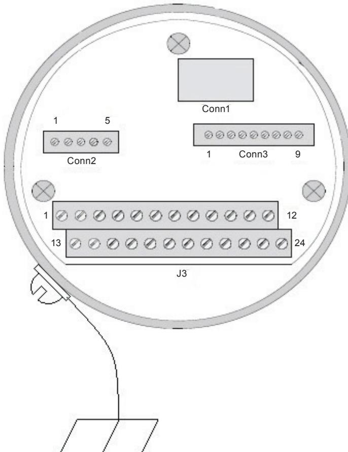
Fig. 18 Enclosure earth ground
