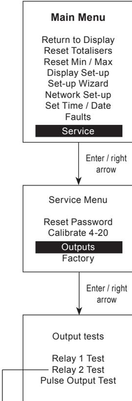
The Relay tests close the selected relay for 3 seconds.
