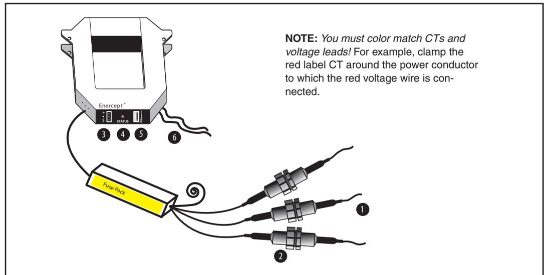
Figure 1 Diagram of typical Enercept meter
