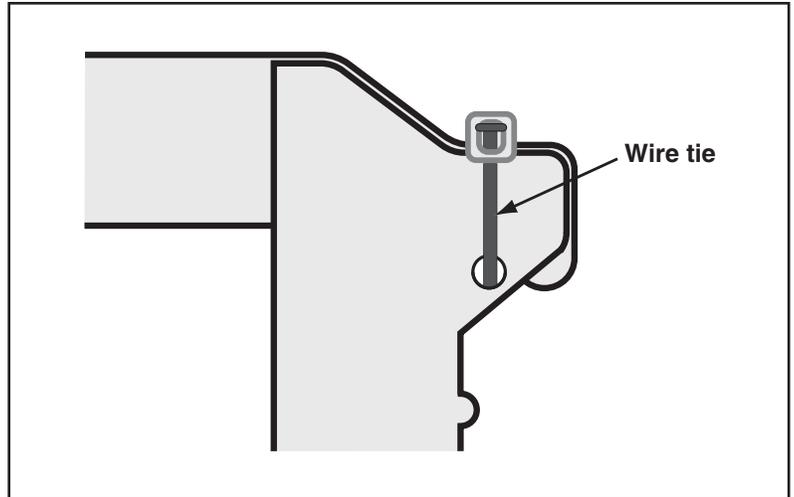
**Figure 7** Wire tie used to secure I-Bar
