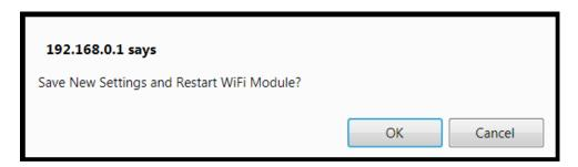
When *OK* is clicked, a confirmation is displayed to indicate configuration is stored in the thermostat's EEPROM. After reboot, the new thermostat credentials will be *admin* for user name and the newly configured Access Point's password for password.
