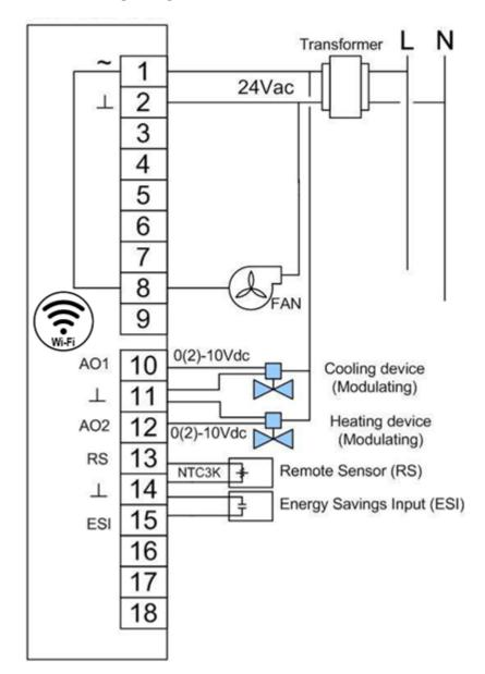
Wiring: 14 to 22 AWG wires or 1.5mm<sup>2</sup> wires.
