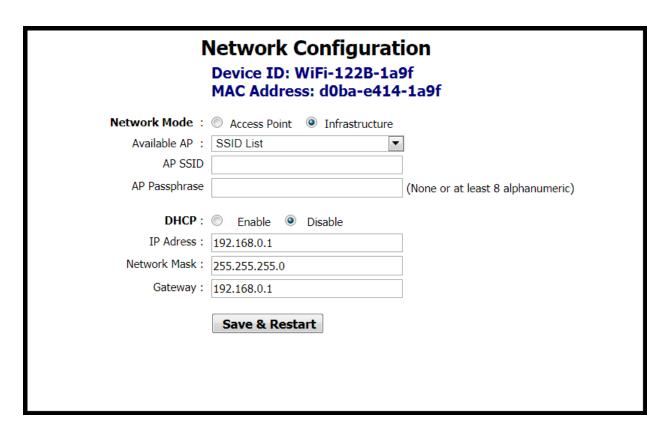
A reboot of the thermostat is required for new IP configuration to take effect. Click the *Save & Restart* button to reboot the thermostat, and you will be prompted to confirm the restart. Click *OK* to Save New Settings and Restart or click *Cancel* to revisit IP configuration.
