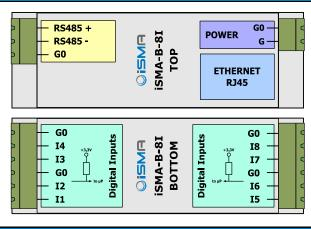
All G0 terminals are connected together internally
