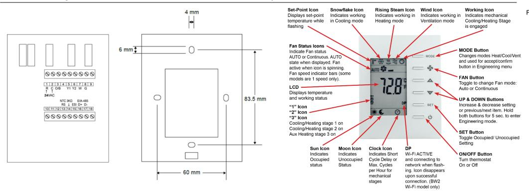
The BASstat has a built-in space temperature sensor with provision for remote wired 3kΩ NTC thermistor sensor, or temperature value can be sent by another device over the BACnet network.
