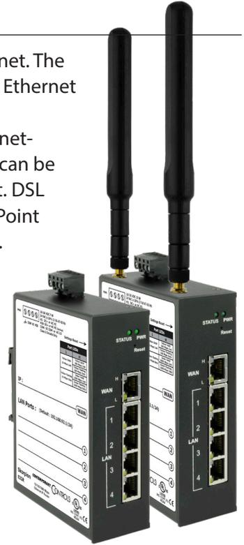
The EIGR-VB and EIGR-C Gigabit IP routers can be configured to operate in OpenVPN server mode as a wired or wireless bridge VPN server for single-site, remote access solutions.
