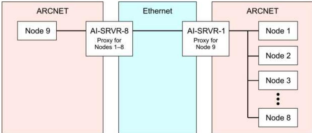
**Figure 10 — AI-SRVR-1 and AI-SRVR-8 Can Work Together**
