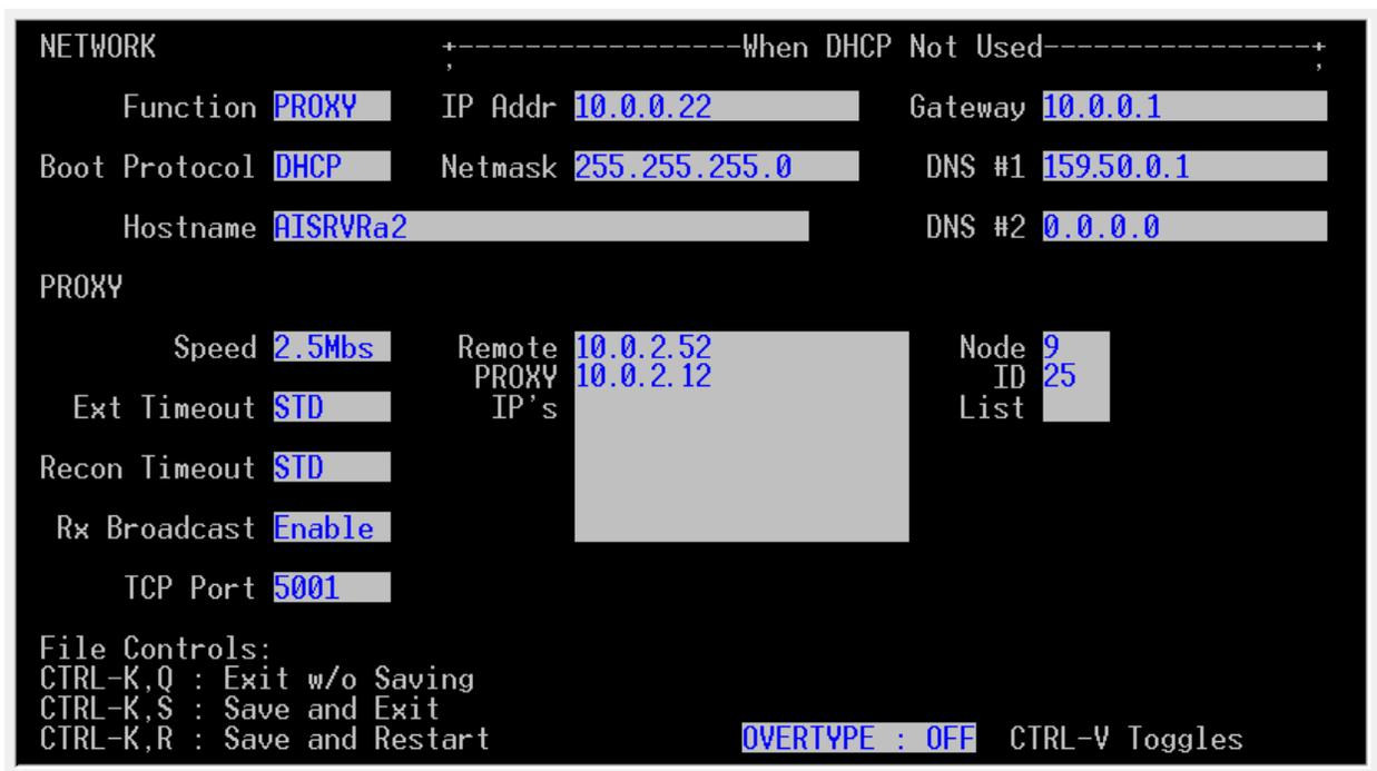
**Figure 13 — Example AI-PROXY Configuration Screen**
