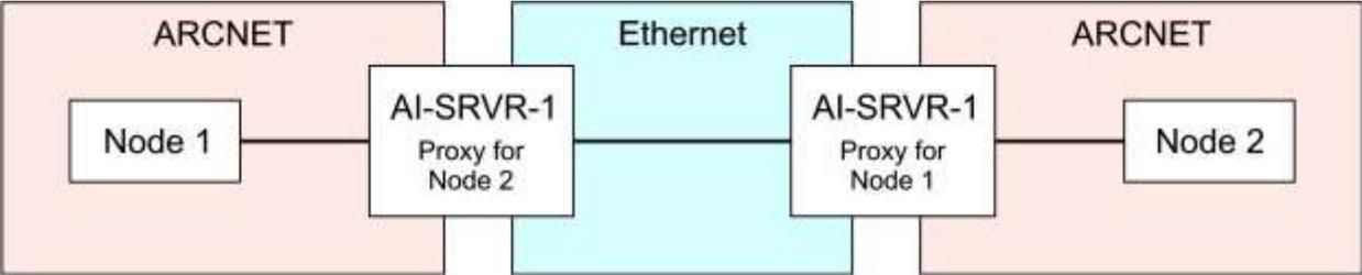
Figure 8 — Each AI-SRVR-1 Can Represent One Node
