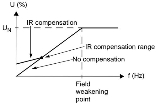
Figure 23 Operation of IR compensation
