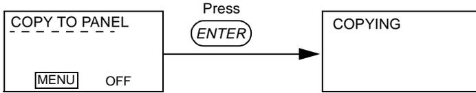
**Note! The drive must be OFF. Parameter 1602 PARAMETER LOCK must be set to 1 (OPEN).**
