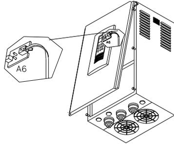
Connect the Control Panel cable to the connector X2, and replace the front cover.
