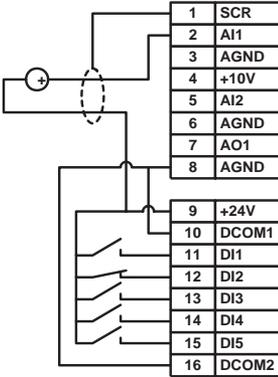
Actual signal (transducer feedback): 0 to 20 mA (PID)
