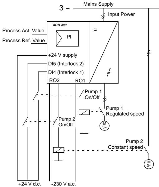
Figure 48 Operation Diagram for the Pump and Fan Control (PFC) Macro. With the default settings, automatic pump alternation is not in use.
