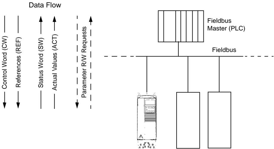
Figure 41 Structure of a fieldbus system.
