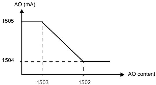
Figure 20 Analog output scaling.
