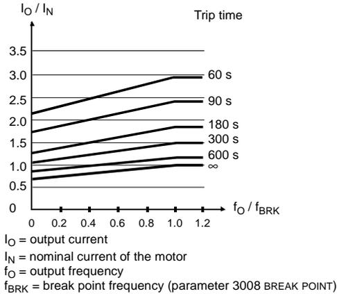
Figure 27 Thermal protection trip times when parameters 3005 MOT THERM TIME, 3006 MOT LOAD CURVE and 3007 ZERO SPEED LOAD have default values.
