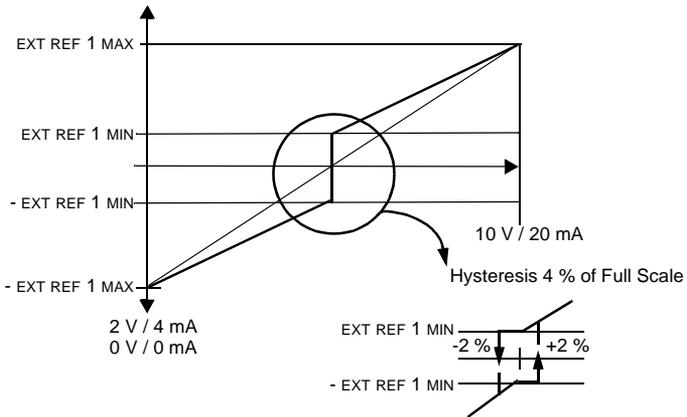
Figure 16 Joystick control. Maximum for external reference 1 is set with Parameter 1105 and minimum with Parameter 1104.
