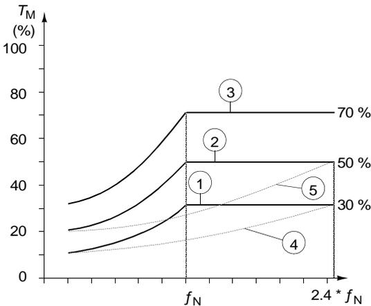
Figure 28 Underload curve types.  $T_M$  nominal torque of the motor,  $f_N$  nominal frequency of the motor.
