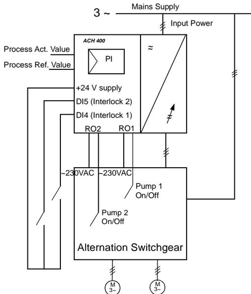
Figure 49 In this example the automatic pump alternation is in use.
