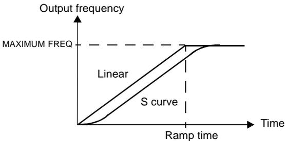
Figure 21 Definition of acceleration/deceleration ramp time.
