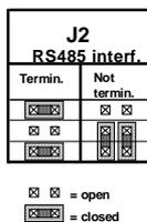
**Note! Ensure that the J2 switch is set for “Not Termin.” on the NIOC card!**
