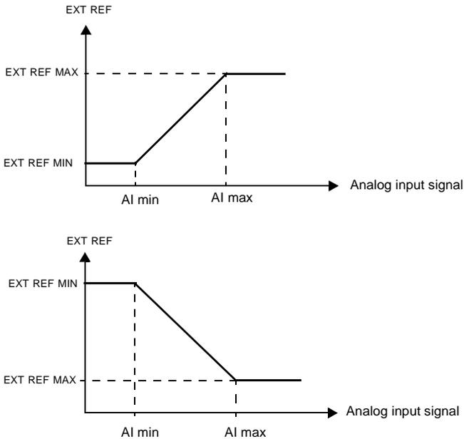
Figure 17 Setting EXT REF MINIMUM and EXT REF MAXIMUM. The range of the analog input signal is set by parameters 1301 and 1302 or parameters 1304 and 1305, depending on the analog input used.
