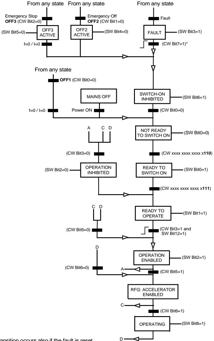
\*This state transition occurs also if the fault is reset from any other source (e.g. digital input).
