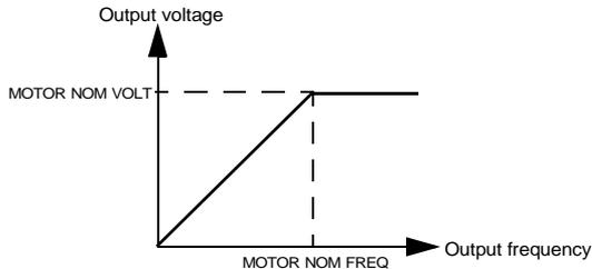
Figure 15 Output voltage as a function of output frequency.
