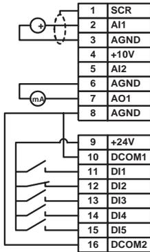
Actual signal (transducer feedback): 0 to 20 mA (PID)
