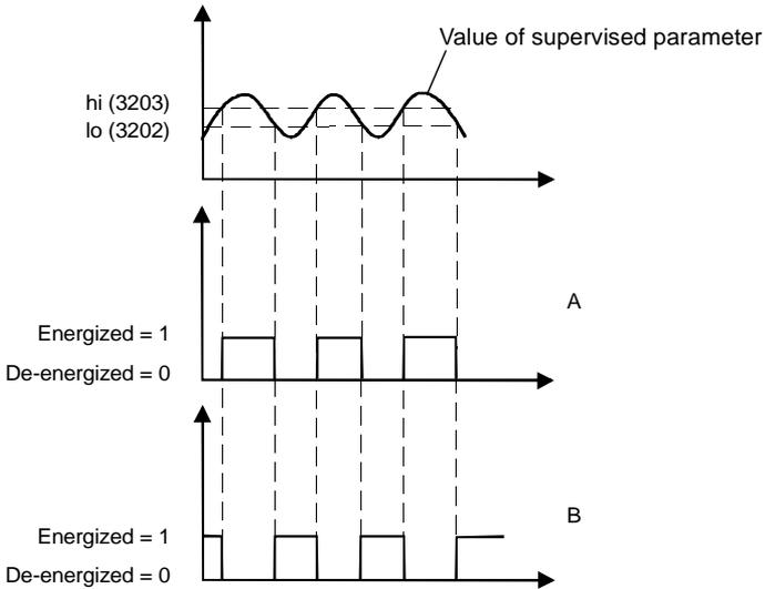
A = Parameter 1401 RELAY OUTPUT 1 (1402 RELAY OUTPUT 2)
