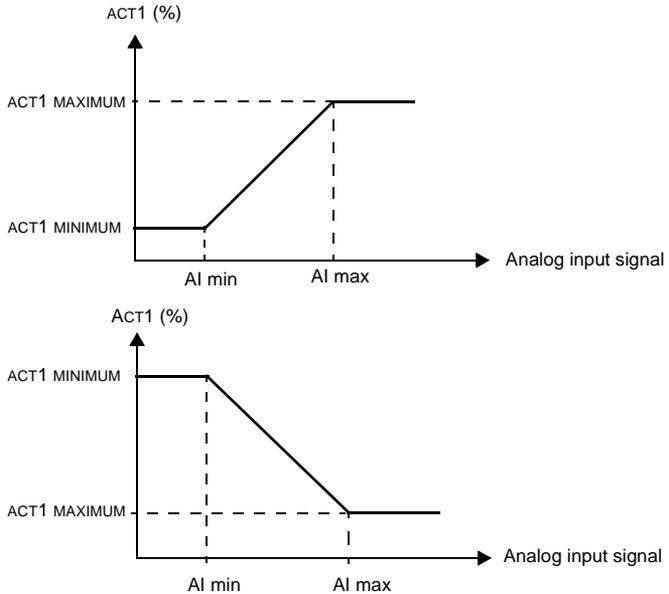
Figure 33 Actual value scaling. The range of the analog input signal is set by parameters 1301 and 1302 or parameters 1304 and 1305, depending on which analog input is used.
