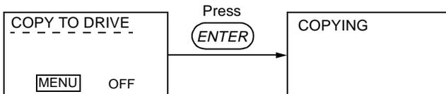
**Note! The drive must be OFF. Parameter 1602 PARAMETER LOCK must be set to 1 (OPEN) and the drive must be in the same macro as the original drive!**
