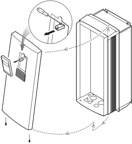
1. Remove the two screws at the lower front edge of the unit and remove the front cover by lifting it carefully from the bottom.
