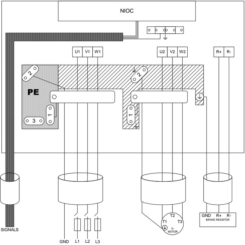
*A view of the recommended wiring configuration.*
