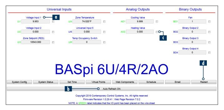
The main web page provides an overview of all real points plus access to other web pages. To configure a point, click on the point name (a) and a configuration page will appear. To observe the updated data for each point, click Auto Refresh button to ON (b). Point values can be temporarily forced by checking the box adjacent to the point
