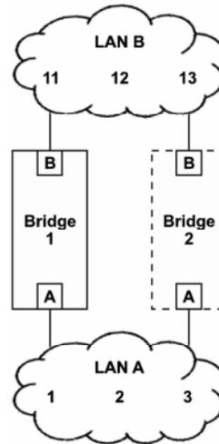
**Figure 1. The addition of Bridge 2 creates a loop.**
