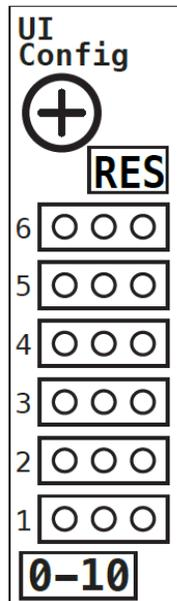
2. For analog, pulse, and binary input (without pull up), set the config jumper to "0-10"
